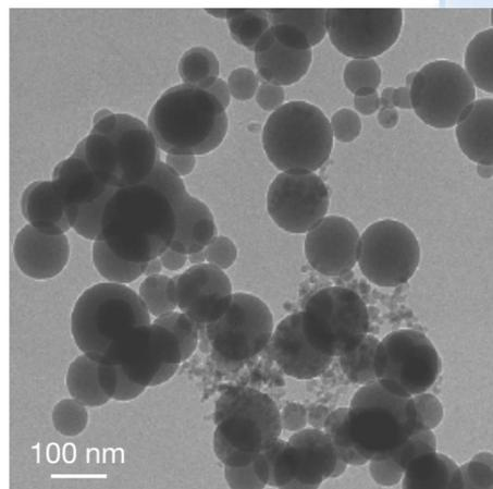
Figure 2 - Non-aggregated, spherical  $\text{SiO}_2$  nanopowder ( $d_{50}=77\text{ nm}$ ) synthesized via flame aerosol technology by ETHZ / EMPA.
