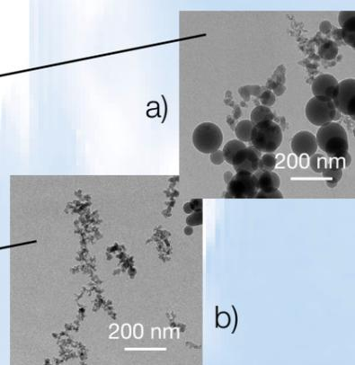
Figure 6 - TEM micrographs of a) non-aggregated, spherical particles and b) fractal-like particles
