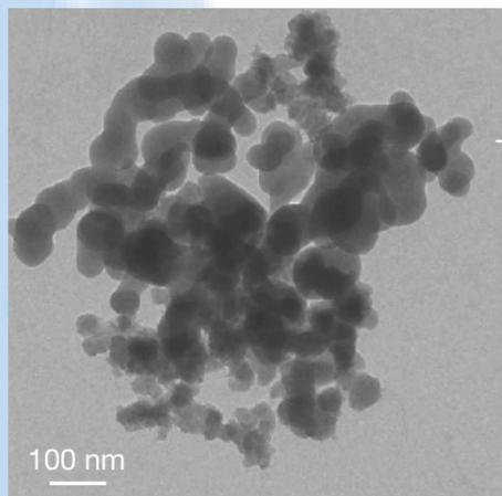
Figure 1 - Commercial  $\text{SiO}_2$  nanopowder (Degussa, Aerosil OX50,  $d_{50}=55\text{ nm}$ ) forming large aggregates
