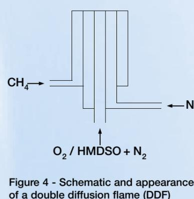
Figure 4 - Schematic and appearance of a double diffusion flame (DDF)
