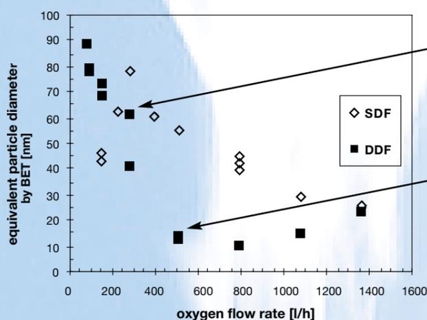
Figure 5 - Correlation of mean particle diameter with oxygen flow rate for a single diffusion flame (SDF) and a double diffusion flame (DDF)
