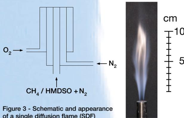
Figure 3 - Schematic and appearance of a single diffusion flame (SDF)
